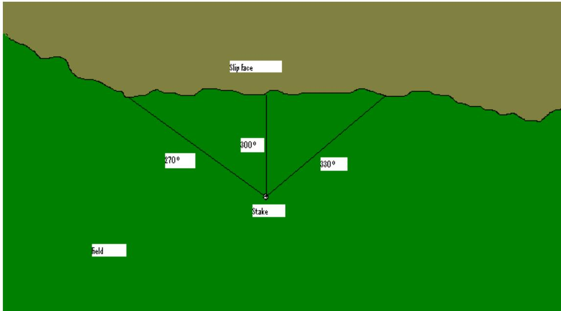
**Figure 14. Possibility for Inaccuracies (note the 270° bearing if measured at 267° could produce a much larger measurement)**
