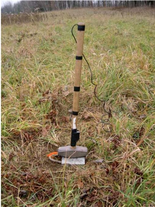
Figure 4. Sledge-hammer with Seismogram Cable (Kanat 2009).
