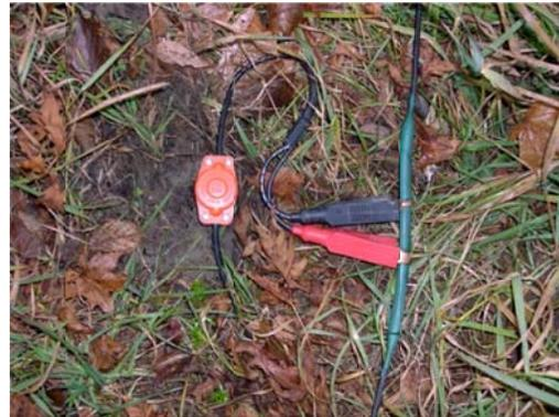
Figure 3. Geophone Detail. (Kanat. 2009)
