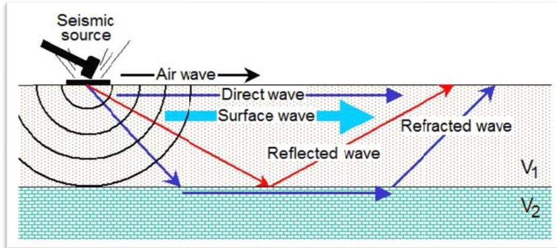
Figure 4. Propagation of Seismic Waves. (Park, 2007).
