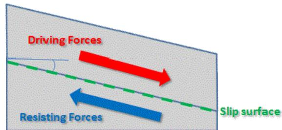
Figure 1. Driving forces vs. Resisting Forces
