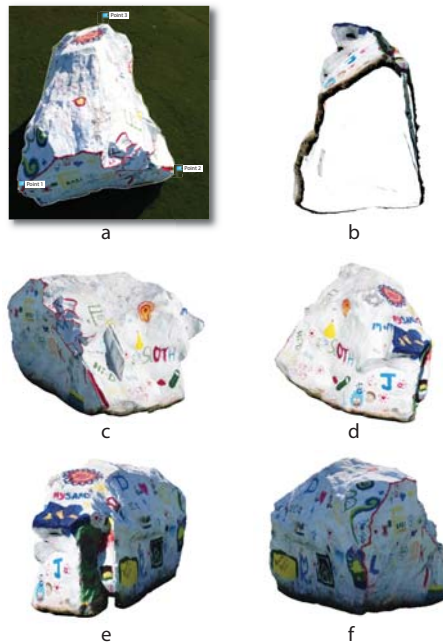
Figure 3. Volumetric calculations for the rock on the campus of JSC. Image 'a' is a photograph taken above the rock and has limits marked. Images 'b-f' are processed. Image 'b' depicts the bottom of rock (never photographed). Images 'c-f' are model representations of the rock rotated ≈90° to the left in each subsequent image (shadows are due to sun angle).
